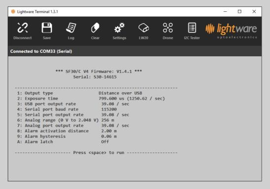
Figure 2:: LightWare Terminal showing menu options
