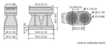
Figure 10 :: Dimension drawings of the SF30
